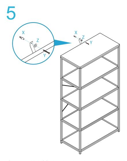
Once assembled lift furniture into place, do not drag. Use a drill to create a small hole lining up with the top of the safety strap (V). Fasten to the wall using 1x washer (Z), 1x wall anchor (X) and 1x wall screw (Y).
