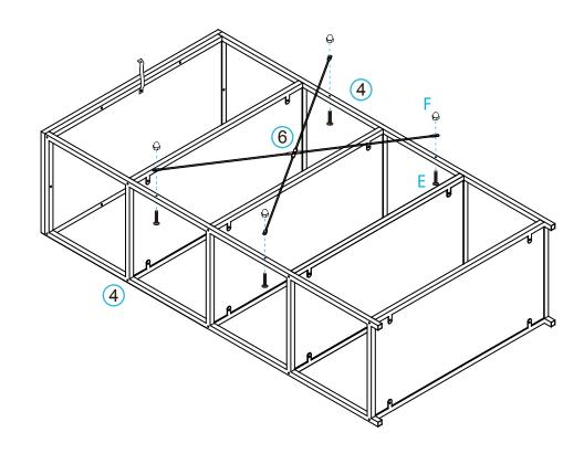
Attach 1x panel [6] to 2x panels [4] secure with 4x bolts (E) and 4x nuts (F). Tighten with a screwdriver.
