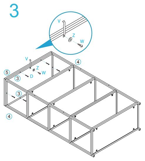
Attach panels [3] and [4] to panel [5] and secure with 6x screws (D). Attach 1x safety strap (V) to the top of the back side of the unit as shown using 1x washer (Z) and 1x screw (W). Tighten with a screwdriver.
